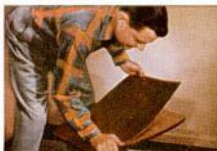
5. Carefully align Formica sheet with edges of table and press down.
